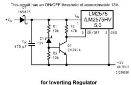
FIGURE 23. Undervoltage Lockout
