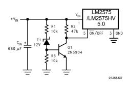
FIGURE 22. Undervoltage Lockout for Buck Regulator
