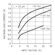
FIGURE 26. Inverting Regulator Typical Load Current
