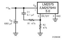
FIGURE 21. Delayed Startup
