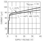
ON /OFF Pin Current (Sinking)
