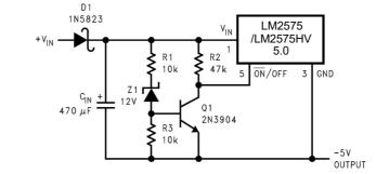
This circuit has hysteresis Regulator starts switching at  $V_{IN}$  = 13V Regulator stops switching at V<sub>IN</sub> = 8V
