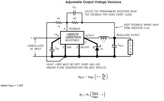
Select R<sub>1</sub> to be approximately 1 k $\Omega$ , use a 1% resistor for best stability. C<sub>IN</sub> — 470  $\mu$ F, 50V, Aluminum Electrolytic Nichicon "PL Series" C<sub>OUT</sub> — 220  $\mu$ F, 35V Aluminum Electrolytic, Nichicon "PL Series" D1 — 5A, 40V Schottky Rectifier, 1N5825 L1 — 68  $\mu$ H, L38 R1 — 1 k $\Omega$ , 1% C<sub>FF</sub> — See Application Information Section
